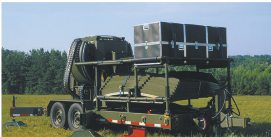
The system shown here features a 16-panel 5.4 meter reflector, a high performance autotracking X-band feed, as well as Y-over-X-axis pedestal configuration.
